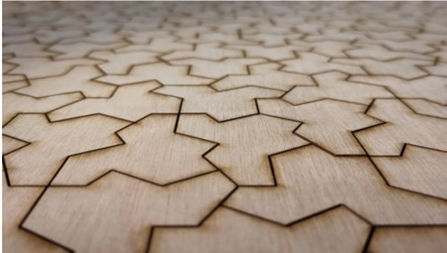
Figure 6.7: Freshly laser-cut copies of the hat, made at the EirLab of Bordeaux INP, January 2025.
