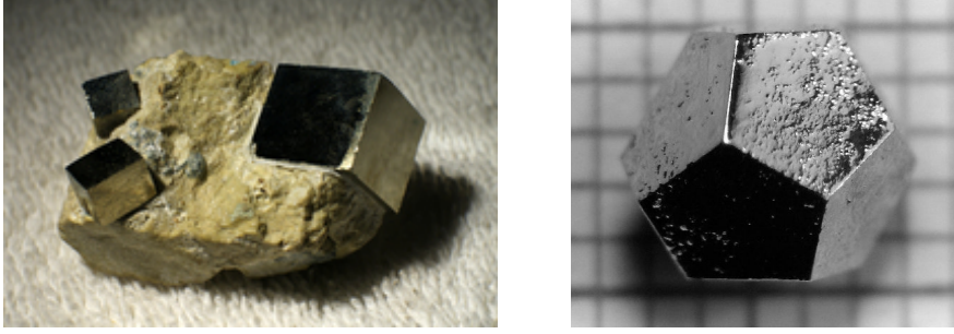
Figure 1.3: Left: A rock containing three crystals of pyrite ( \text{FeS}_2 ). The crystal structure of pyrite is primitive cubic, and this is reflected in the cubic symmetry of its natural crystal facets. Right: A Ho-Mg-Zn dodecahedral quasicrystal formed as a pentagonal dodecahedron. Unlike the pyrite, the quasicrystal has faces that are regular pentagons. Image credits: https://en.wikipedia.org/wiki/Cubic_crystal_system and https://en.wikipedia.org/wiki/Quasicrystal .
